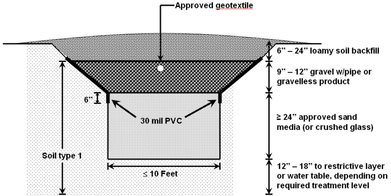
**Figure 3 - Reaching More Suitable Soils at a Depth Greater Than 3 Feet**
