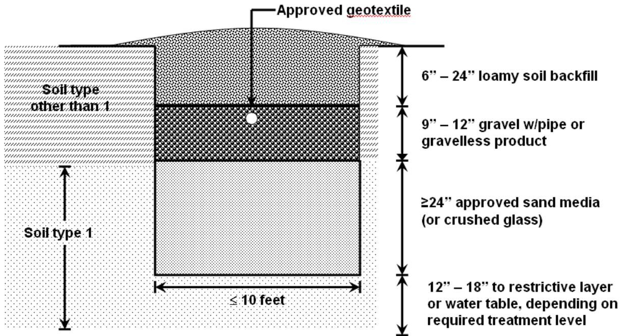
**Figure 2.2 - Type 1 Soil Extending up into Trench/Bed Zone (Option 1)**
