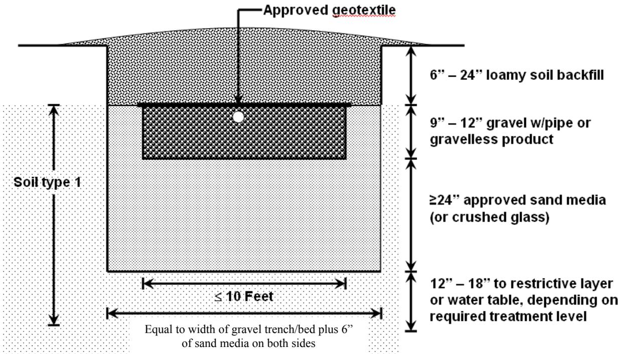
**Figure 2.3 - Type 1 Soil Extending up into Trench/Bed Zone (Option 2)**
