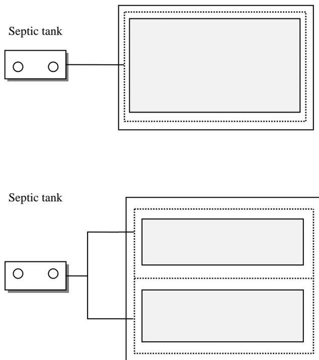
**Figure 4- Drainfield Layout With D-Box**
